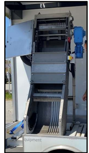
Aqualtec "Raketec" Bar Screen for Main Pump Station.
